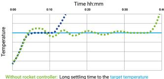
Without rocket controller With rocket controller:
