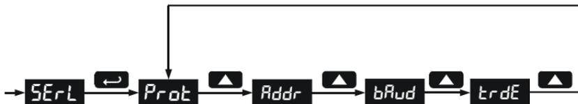
When using more than one meter in a multi-drop mode, each meter must be provided with its own unique address. The address may be programmed from 00 to 99 for PDC protocol and from 1 to 247 for Modbus<sup>®</sup> protocol. The transmit delay may be set between 0 and 199 ms.
