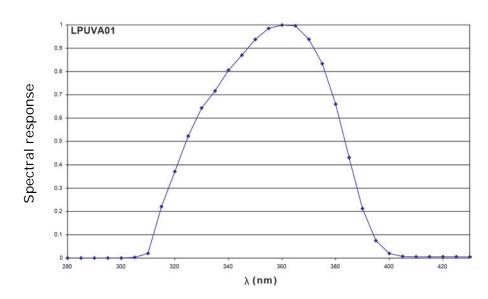
The calibration is performed by reference to our primary standard with monochromatic light at 365 nm obtained separating the emission line of a Xe-Hg lamp with an inferential filter. To get best performances from your LPUVA01 it is strongly recommended that the calibration be checked annually. The temperature has a negligible influence on the spectral response of the probe.
