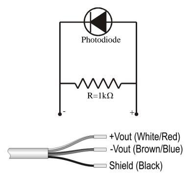
To obtain a reading precision of 1% of the difference in potential at the ends of the resistance, the probe must be connected to a digital multimeter with input resistance > 100  $k\Omega$
