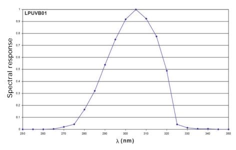
Probe calibration is carried out by using a 313 nm line of a Xe-Hg lamp, filtered through a special interferential filter. Measurement is carried out by comparison with the primary standards, assigned to Delta OHM Metrological Laboratory.
