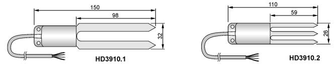
Fig. 1: dimensions (mm)
