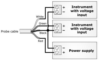
Fig. 4: analog outputs connection
