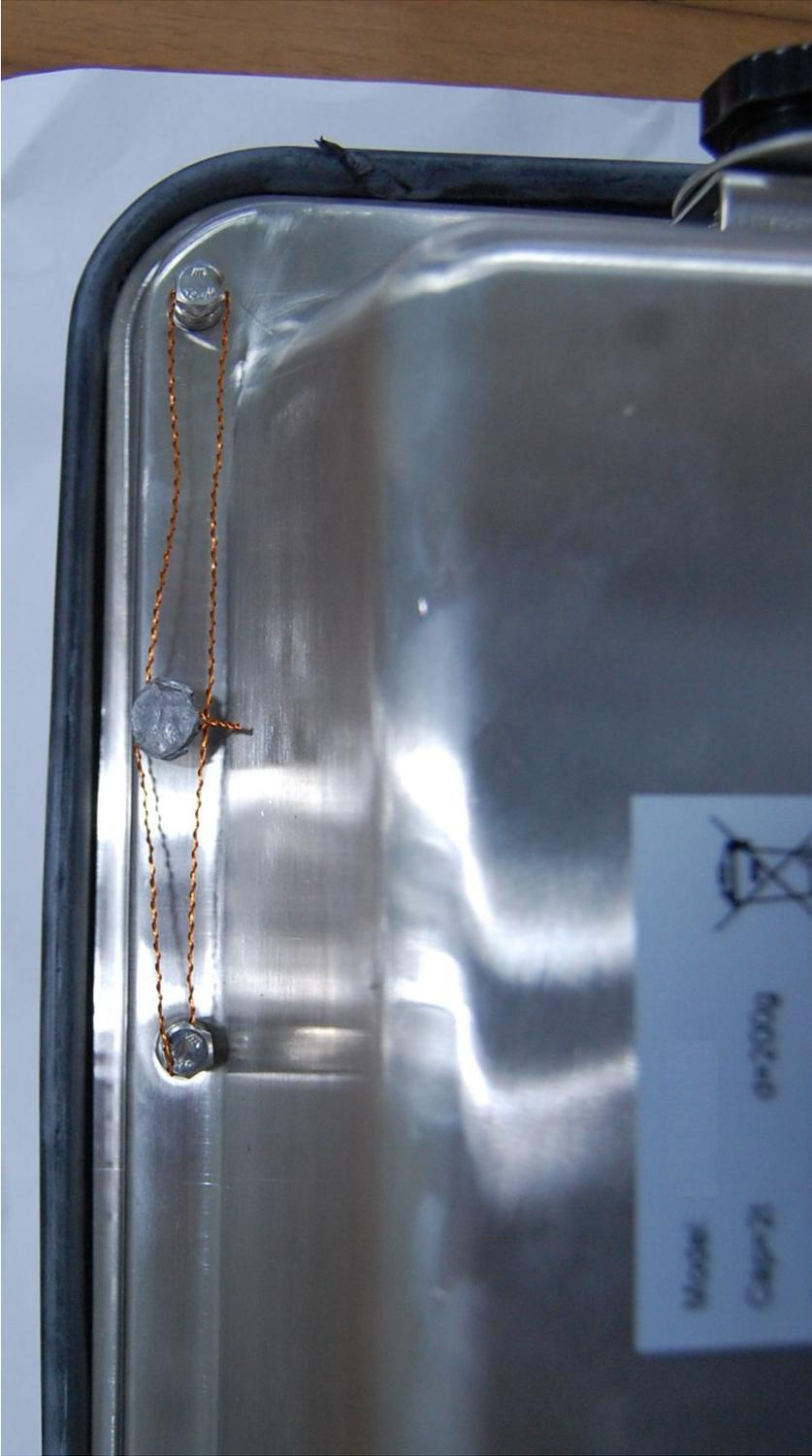
**Figure 4** Sealing of KFN-TM / SFB / UFN / BFN / NFN.
