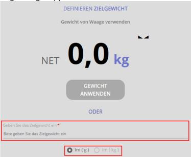
Enter the target weight and select the weighing unit: **Here is an example:**
