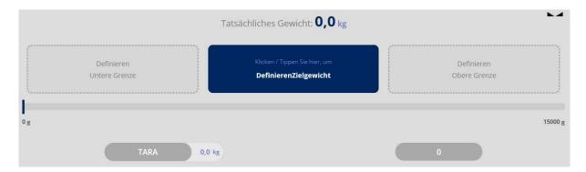
If necessary, place a tare container on the weighing plate and tare with button TARE:
