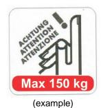
⇒ Do not exceed the permissible rated load of the crane (overhead crane), crane scale or any components used to hoist the load on the crane scale.
