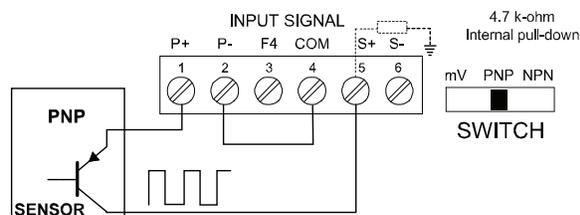
**Figure 16: PNP Sensor Powered by Internal Supply**
