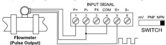
**Figure 12: Flowmeter Powered by Internal Power Supply**
