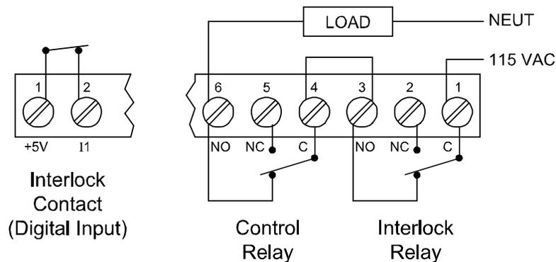
**Figure 26: Interlock Connection**
