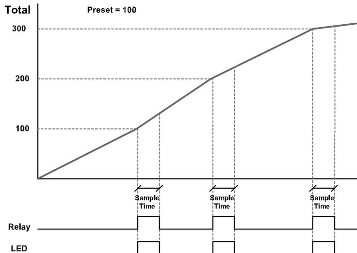
When the batch total reaches the set point, the relay trips and the sample time starts. After the sample time has elapsed, the relay resets. The cycle repeats every time the set point value is added to the batch total.
