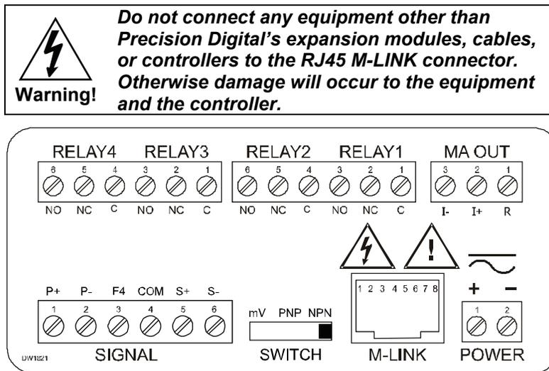
**Figure 10: Connector Labeling for Fully Loaded PD6310**
