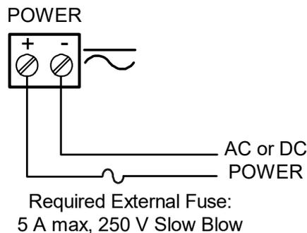
**Figure 11: Power Connections**
