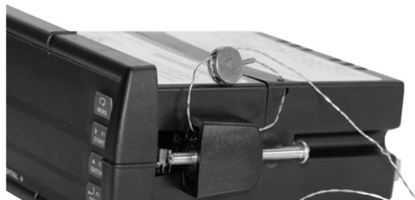
**Figure 9: Close and Crimp Seal Wire Security Loop**
