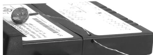
**Figure 7: Wire Loop through Rear Case Pass-Through**
