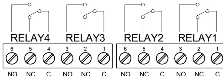
**Figure 18: Relay Connections**
