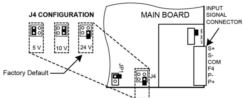
**Figure 4: Transmitter Supply Voltage Selection**
