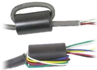
Figure 1-4: Installing the Ferrite Core
