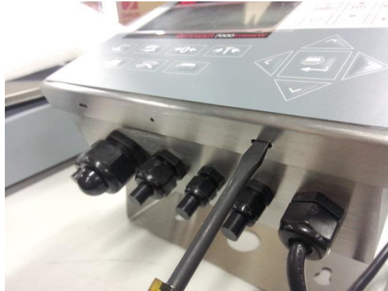
Figure 1-2: Opening the Harsh Enclosure
