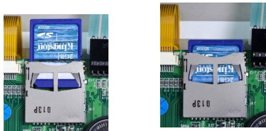
Figure 1-10: Sliding an SD Card into the SD Socket (left); SD Card Installed (right)
