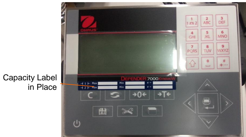
Figure 1-12: Capacity Label Installed
