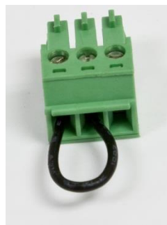
Figure 5-4: Jumper Wire Between COM1 Transmit and Receive Indicators
