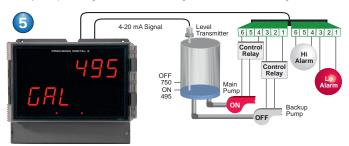
Relay #1 trips the Low Level Alarm at 495 gallons and resets at 750 gallons.
