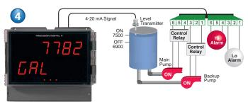
Relay #2 trips the High Level Alarm at 7500 gallons and resets at 6900 gallons.
