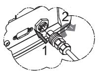
Note: To connect T24PE to other bases, a loadcell connector needs to be soldered as shown above.
