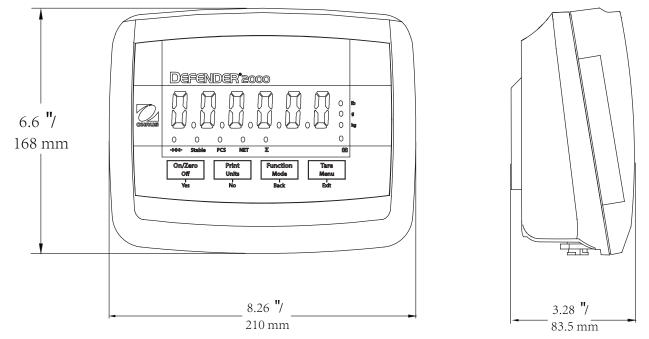
Figure 8-1. Indicator Overall Dimensions.
