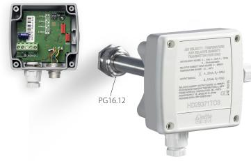
In the TO version, the duct probe is fixed to the electronics enclosure and it is available in three different lengths. To fix the probe to the duct, you can use, for example, the HD9008.31... flanges, a 3/8" universal biconical connection or the PG16... metal cable glands (Ø10...14 mm).
