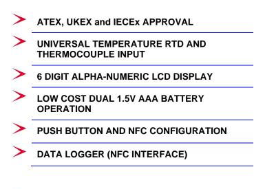
The DM650XTM battery powered temperature indicator accepts RTD or thermocouple temperature sensors and displays the sensor temperature in °C, °F or K on a 6-digit LCD display. Configuration is achieved by operating a single push button and navigating a menu structure. A contactless NFC interface is also provided for configuration and the data logger function.
