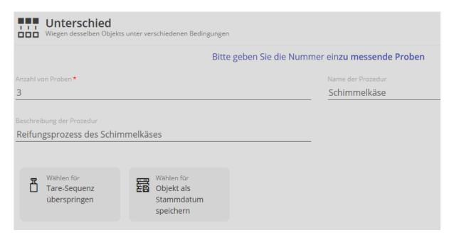
If the weight of the tare container is known, click the field "Skip tare sequence". In the field a small hook appears and the line to enter the tare weight appears. Enter tare weight:
