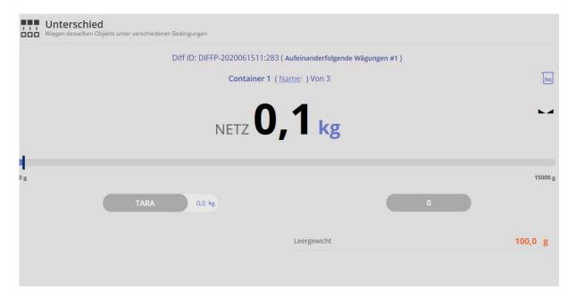
In order to determine the start weight of the second sample, remove sample 1 and place sample 2 and click CONTAINER 2.
