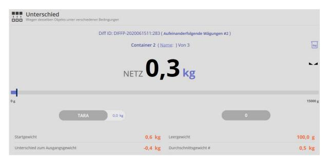
In order to determine the start weight of the third and last sample, remove sample 2 and place sample 3 and click CONTAINER 3. Finish the process with SAVE and save.
