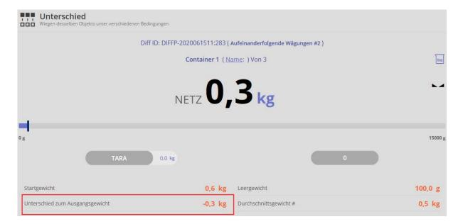
In order to determine the start weight of the second sample, remove sample 1 and place sample 2 and click CONTAINER 2.
