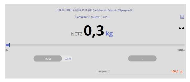
To determine the start weight of the third and last sample, remove sample 2 and place sample 3 and click SAVE.
