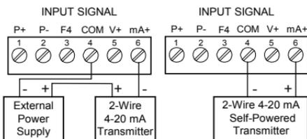
Wiring for a 4-20 mA input using internal power supply.
