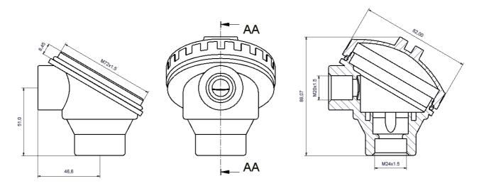
Material Aluminium Alloy **Protection IP68** Mounting Sensor only
