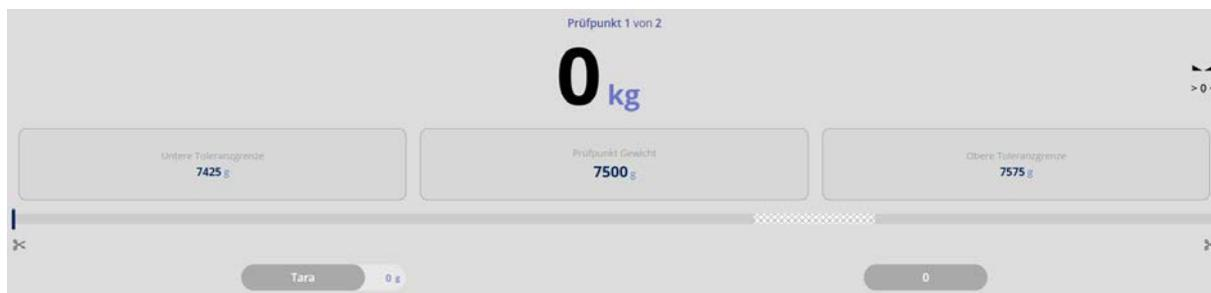
Now the first test point can be set. Load the balance until the green bar graph appears:
