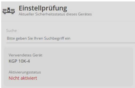
Click the field, the device information and the input fields for the adjustment test will appear. Enter the last adjustment and the time interval:
