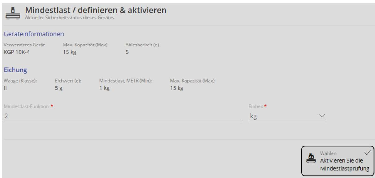
Finish the process with the blue button „Save“ bottom right. If the weight on the weighing plate below this value, the balance will be blocked.
