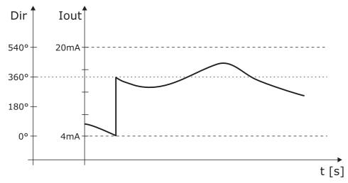
If 539° value is exceeded in extended mode, the output goes to the value corresponding to 180°.
