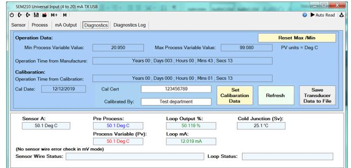
The diagnostic log tab can be set to record a log onto the SEM210. A 150 point rolling log set at time intervals between 5 s up to 1 hr can be recorded for viewing or can be saved to a text file.
