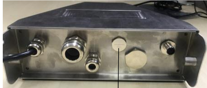
Figure 2-5 Strain Relief for Option
