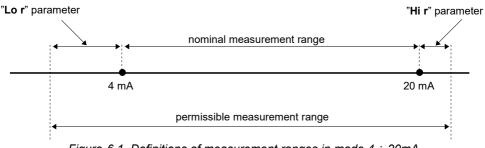
Figure 6.1. Definitions of measurement ranges in mode 4 ÷ 20mA
