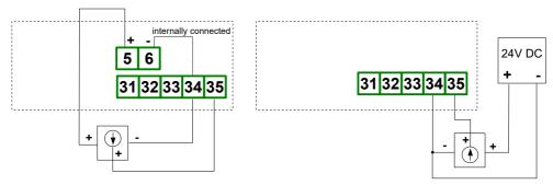
Figure 4.13. Connection of voltage transducer
