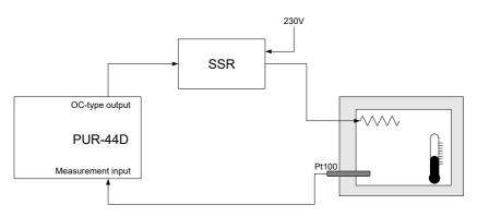
Figure. 10.5 Example arrangement of connections for auto-tuning
