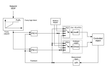
Figure 6.5. The general structure of the PUR-44D device
