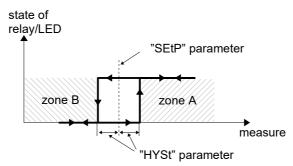
Figure 6.10. One threshold control of the relay/LED outputs
