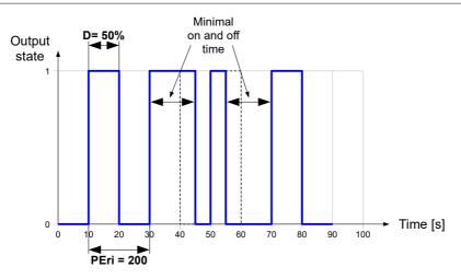
Figure 6.15. An example of the progress of an OC type PWM output signal in PULS mode
