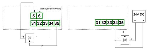
Figure 4.12. Connection of 3-wire current transducer
