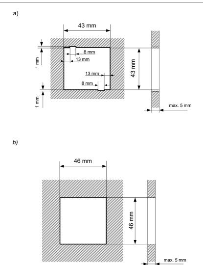
Figure 4.1. Mounting hole dimensions: a) recommended b) allowable
