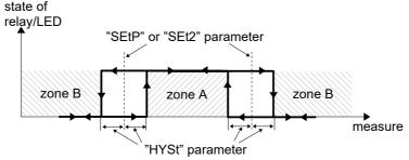
Figure 6.11. Two threshold control of the relay/LED outputs
