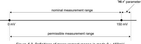
Figure 6.2. Definitions of measurement ranges in mode 0 ÷ 150mV
