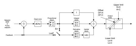
Figure 7.2. General diagram of the PID controller featured in the PUR-44D device
