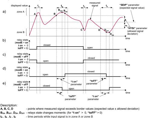
Figure 6.12. Principle of LED/relay output operation for one threshold mode
