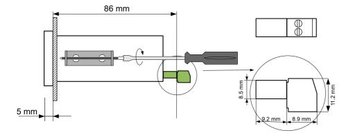
Figure 4.2. Installing of brackets, and dimensions of connectors.
