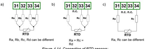
Figure 4.14. Connection of RTD sensors: a) 4-wires circuit; b) 3-wires circuit; c) 2-wires circuit
