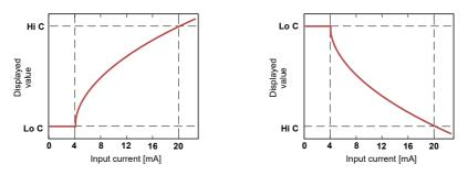
Figure. 10.3 Normal ("Lo C" < "Hi C) and inverted ("Lo C" > "Hi C) characteristic
