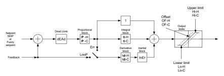
Figure 6.6. General scheme of the PID controller implemented in the PUR-44D device
