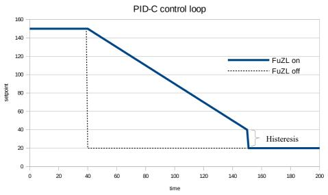
Figure 6.9. Comparison of the PID-C controller's response to a change in the setpoint using and without the use of fuzzy logic
