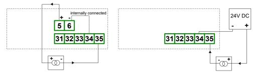
Figure 4.11. Connection of 2-wire current transducer
