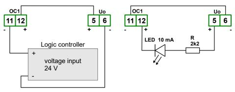
Figure 4.17. Example of OC-type outputs connection (for device with OC-type output only)
