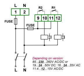
Figure 4.15. Connection of power supply and relays
