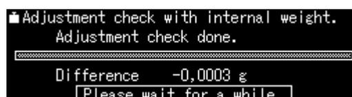
Adjustment check with internal weight.
