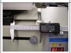
Move the slider to the left until the distance is approximately 100 mm. Don't care about the exact distance, you can input the caliper reading into the software to fix the calibration
