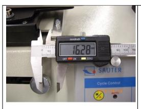
Move the slider to the right until the limit switch stops the movement. Take a caliper and measure the distance between the slider and the holder from the LD length meter. If possible zero the caliper.
