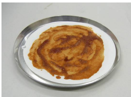
Distributed evenly at a fiber glass filter
