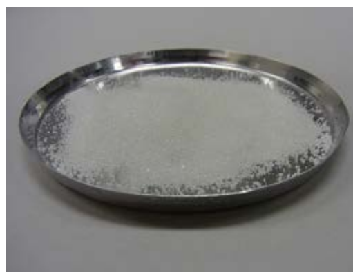
No discoloration, but surface slightly solidified.
