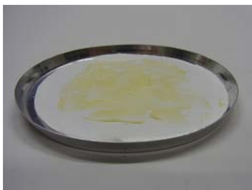
Sample distributed evenly by a spatula at a fiber glass filter
