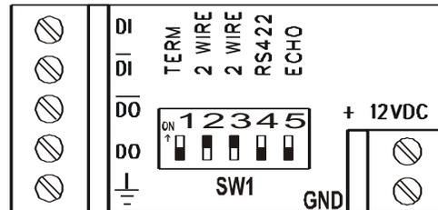
**Figure 13. PDA7485 Terminal Connectors and DIP Switch**
