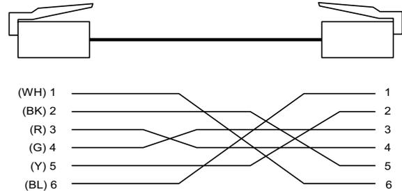
**Figure 11. Standard Modular Cable Wiring**
