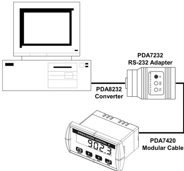
**Figure 23. Connections for PDA8232 to serial device**
