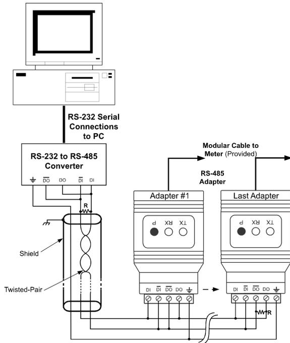
**Figure 15. RS-485 Two-Wire Multi-Drop Wiring**
