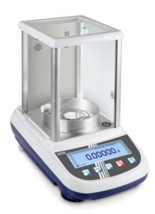
**KERN ALJ 200-5DA** with optional ionisor **■**, see Accessories. High-precison semi-microbalance. Thanks to its precison, this model is suitable to calibrate pipettes.
