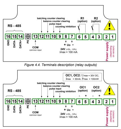
Figure 4.5. Terminals description (OC-type outputs)
