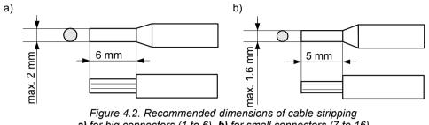
a) for big connectors (1 to 6), b) for small connectors (7 to 16)
