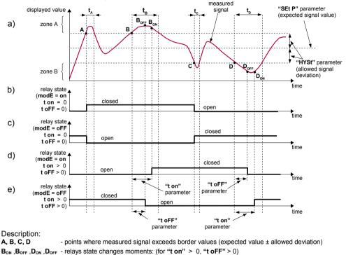
$\mathbf{t}_{A}$ ,  $\mathbf{t}_{B}$ ,  $\mathbf{t}_{C}$ ,  $\mathbf{t}_{D}$  - time periods while input signal is in zone A or zone B
