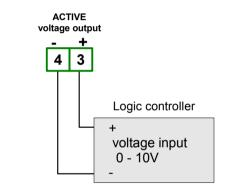
Figure 4.18. Example of active voltage outputs connection (for device with active voltage output only)
