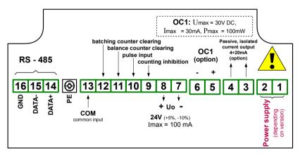
Figure 4.9. Terminals description (OC-type and passive current outputs)
