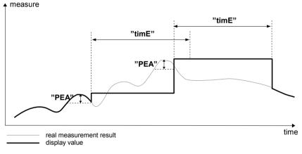
Figure 6.2. Process of peaks detection
