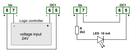
Figure 4.15. Example of OC-type outputs connection
