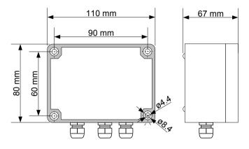
Figure 4.1. Device and assembly dimensions
