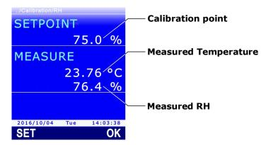
Fig. 13.3.5: calibration at 75%RH
