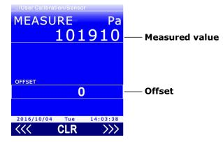
Fig. 13.1.1: barometric pressure calibration
