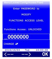
5. The instrument returns to the ACCESS PSWD item. The indication of the protected status appearing at the end of the menu item list is updated to the new status. Press **ESC** twice to exit the menu.
