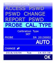
*Note*: if a user calibration is not available for the probe, the default setting is AUTO and cannot be changed.
