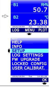
3. Select the **AUTO SWITCHOFF** item using  $\blacktriangle$  and  $\blacktriangledown$ , then press the F3 key (OK command) to confirm.
