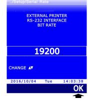
5. The instrument returns to the SERIAL RATE item, Press **ESC** twice to exit the menu.
