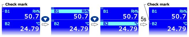
Fig. 3.1.1: selecting a measurement line
