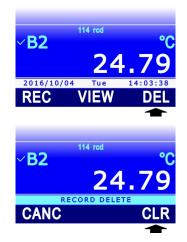
To disable the RECORD function, select instead the **CANC** command by pressing the F1 key. Press **ESC** to return to the previous menu level.
