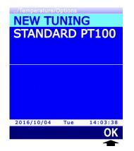
Fig. 13.3.2: types of calibration for the temperature sensor
