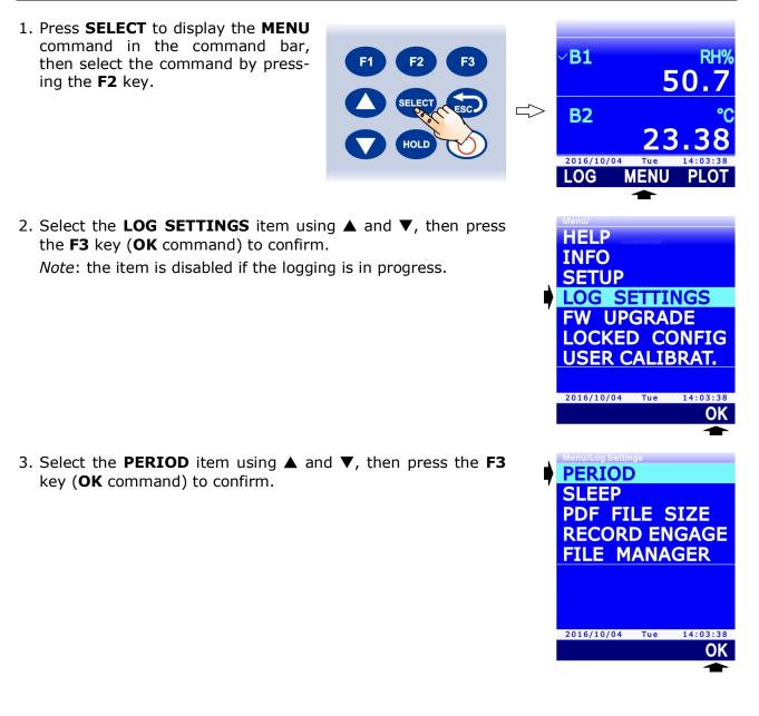
Using ▲ and ▼, select the interval for the automatic logging or the "MANUAL" item to set the manual logging.
