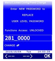
5. The instrument returns to the PSWD CHANGE item, press **ESC** twice to exit the menu.
