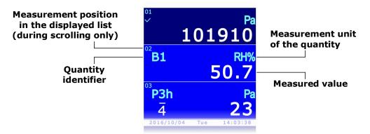
Fig. 3.2: measurements display
