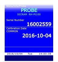
Fig. 11.2: information concerning the connected probe
