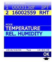
Fig. 13.3.1: selecting the sensor to be calibrated
