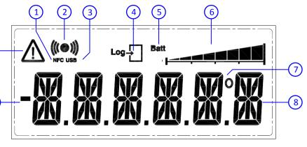
1. NFC - The Symbol is on when a NFC field is detected. When a detected field is lost the symbol will turn off after a few seconds.
