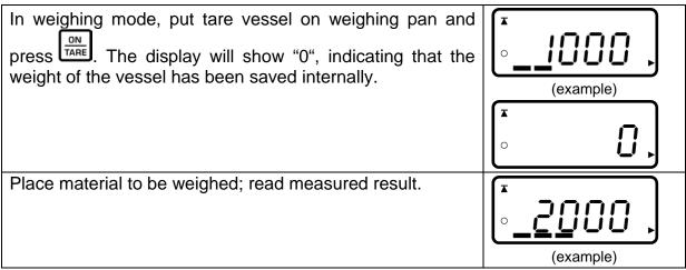
If one after finishing the weighing process presses again the TARE button, "0" appears anew in the display.
