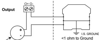
CSA Entity Certified device installed per manufacturer's Hazardous Location Installation Drawing.
