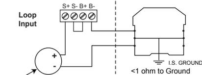
ATEX Entity Certified transmitter installed per transmitter manufacturer's Hazardous Location Installation Drawing.
