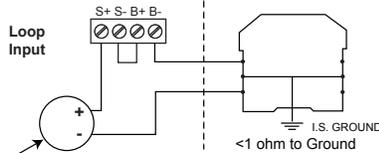
CSA Entity Certified transmitter installed per transmitter manufacturer's Hazardous Location Installation Drawing.
