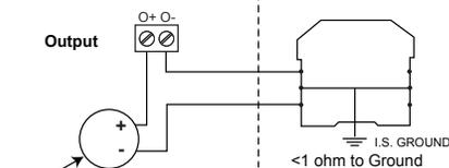
ATEX Entity Certified transmitter installed per manufacturer's Hazardous Location Installation Drawing.
