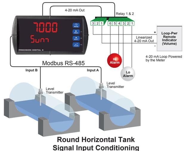
Round Horizontal Tank Signal Input Conditioning
