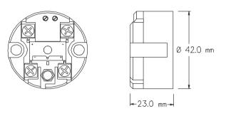
Mounting holes : 2 holes 5.5mm diameter, 33mm centres
