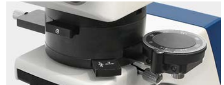
Bertrand lens, \lambda Slip, 360° rotatable analyser (removable)
