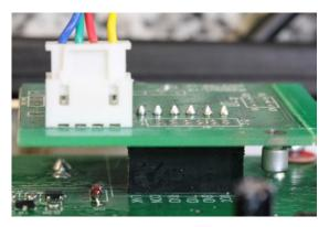
Plug cable into the RS-232 board
