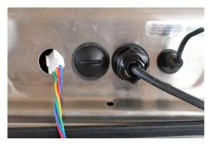
Guide the interface cable through the opening of the terminal
