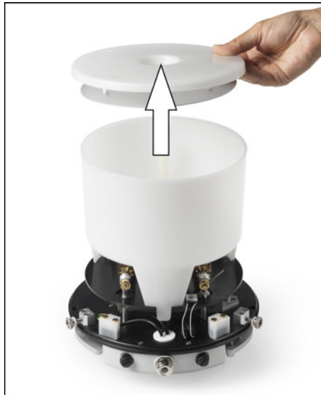
Fig. 9.3: rainfall collecting reservoir
