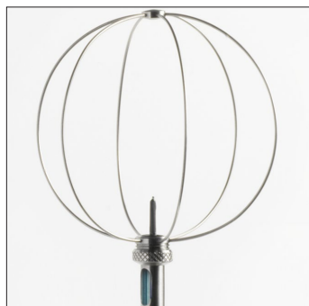
Fig.2 hot-wire probe mod. HD2001.2.
