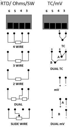
RTD input wires must be equal length and type.
