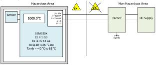
Sensor wires must be isolated from earth, breakdown voltage 500 V dc
