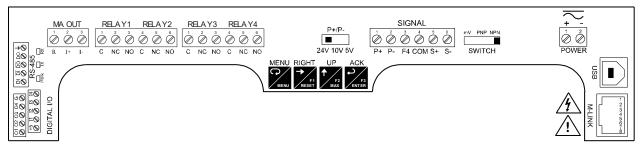
Figure 7. Connector Labeling for Fully Loaded PD2-6300
