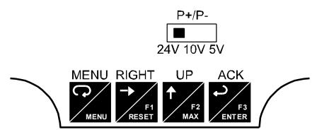
Figure 6. Transmitter Supply Voltage Selection
