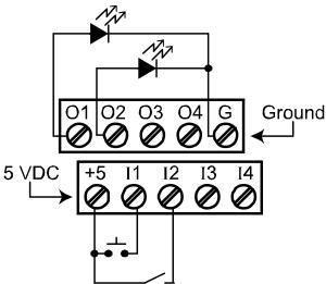
Figure 22. Digital Input and Output Connections
