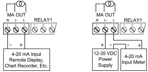
Figure 24. 4-20 mA Output Connections
