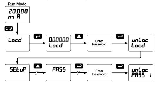
If the correct six-digit password is entered, the meter displays the message unlocked) and the protection is disabled until a new password is programmed.
