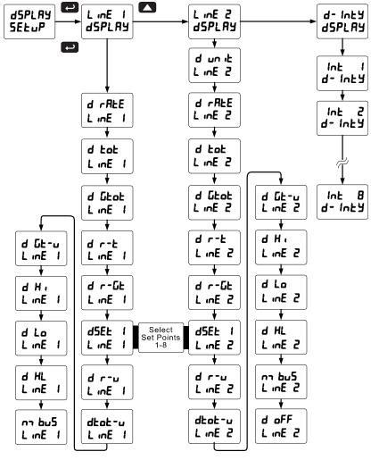
**Display Intensity:** The meter has eight display intensity levels to give the best performance under various lighting conditions. Select intensity 8 for outdoor applications. The default intensity setting is 8.
