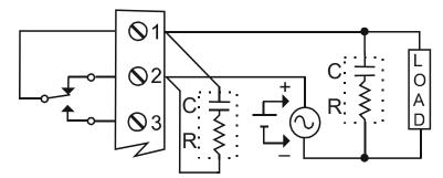
Figure 16. AC and DC Loads Protection
