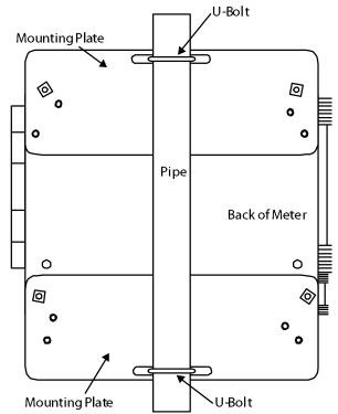
Figure 4. Vertical Pipe Mount Assembly
