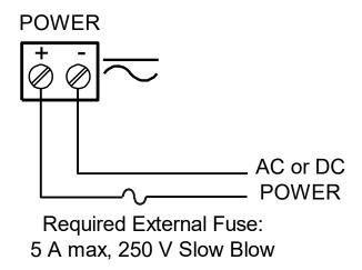
**Figure 8. Power Connections**
