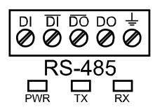
The RS-485 connector has three diagnostic LEDs: a Power (PWR)
