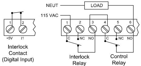
Figure 25. Interlock Connections
