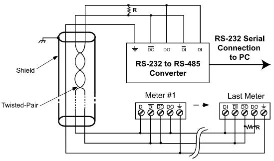
Figure 19. RS-485 Two-Wire Multi-Drop Wiring
