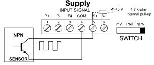
Figure 12: NPN open Collector Input
