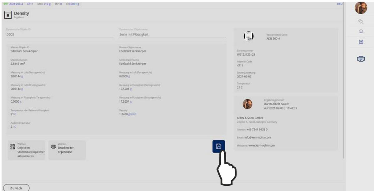
After saving the balance automatically returns to density determination mode. A new density determination can be started.
