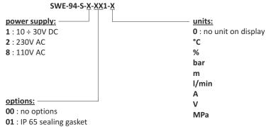
08: operating temp.  $-20^{\circ}\text{C} \div +50^{\circ}\text{C}$
