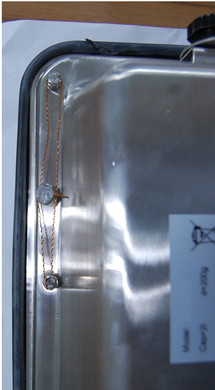
Figure 4 Sealing of KFN-TM / SFB / UFN / BFN / NFN. (method B)
