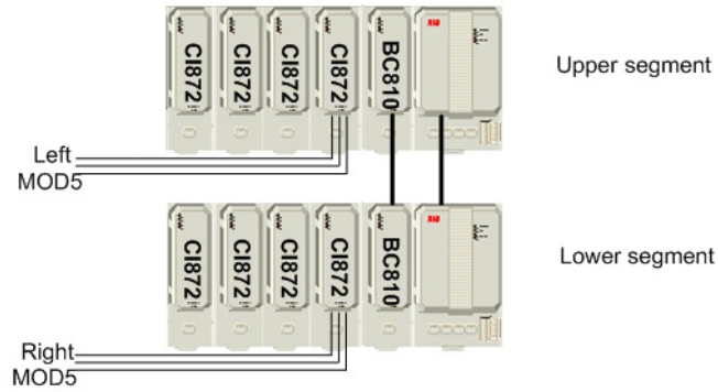
Figure 36. Maximum Configuration Using PA Controller
