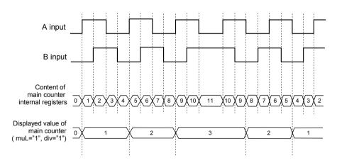
Figure 6.1. The counting principle of the **SLK-94T** counters
