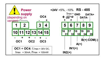
Figure 4.6. Terminals description (OC-type outputs)
