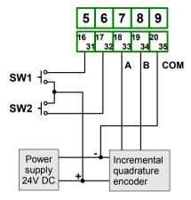
Figure 4.11. An example connection of incremental encoder.
