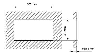
Figure 4.2. Allowable mounting hole dimensions
