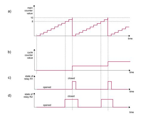
Figure 6.6 Example of relay controlling in "standard" mode; settings: "SEtP 1"=10, "SEtP 2"=8, "ArESEt"="on", "timE 1">0, "timE 2">0
