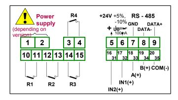
Figure 4.5. Terminals description (relay outputs)
