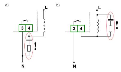
Figure 4.9. Examples of suppression circuit connection: a) to relay terminals; b) to the inductive load
