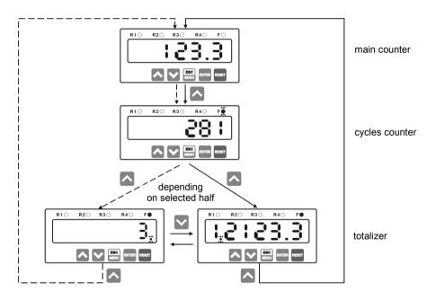
Figure 6.4. Examples of switching between counters
