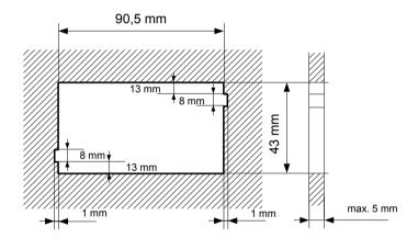
Figure 4.1. Recommended mounting hole dimensions
