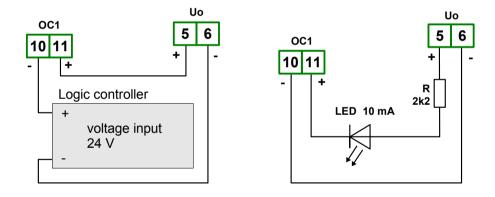
Figure 4.10. Example of OC-type outputs connection
