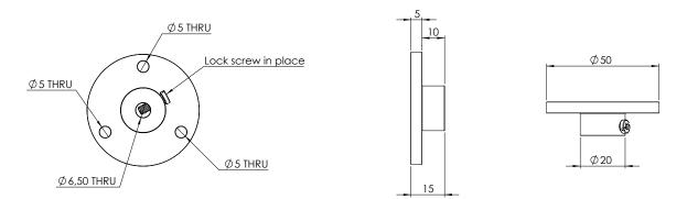
For Ø15mm, Ø22mm or Ø32mm sensor element, cast steel, bolt fitting only, no counter flange
