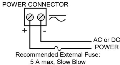
Figure 9. Power Connections
