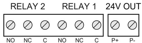
Figure 12. Relay & 24 V Output Connections
