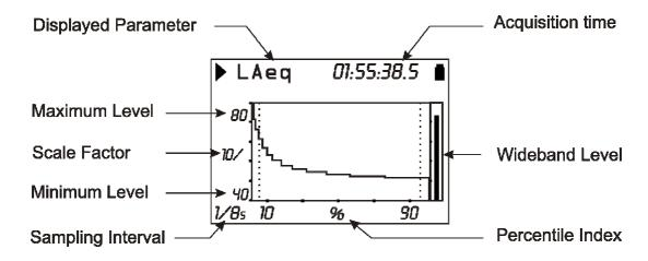
Fig. 7 - Description of the percentile level display
