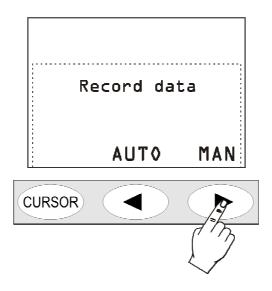
If the *manual* recording has been selected, the instrument will behave as per the above description (Single record recording).
