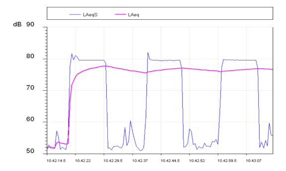
In the measurement time span, the Leq Short (LAeqS) shows three phases with high noise, about 80dB, and a variable 52-60dB background noise.
