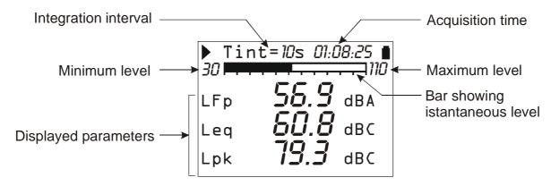
The "analogue bar" shows the unweighted sound pressure instantaneous level in an 80 dB interval.
