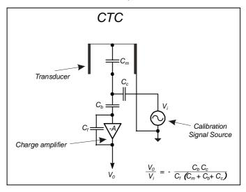
ment. The electric calibration adjusts the acoustic response of the microphone-sound level meter chain, both for wideband channels, and for those with a constant percentage bandwidth. In case of continuous instrument drifts, it is suggested to carry out an acoustic calibration to verify that there are no other problems both in instrument and microphone.
