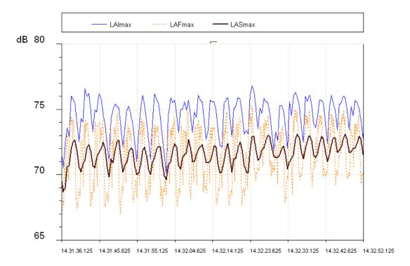
In case a sound source emits noises with a strong impulsive component, the level measured with the IMPULSE constant will be much higher than the SLOW level. The figure shows the sound level profile, measured simultaneously using the FAST, SLOW, and IMPULSE time constant by a surface mount machine.
