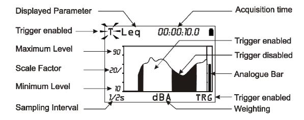
Fig. 9 - Description of the "Event trigger - display"
