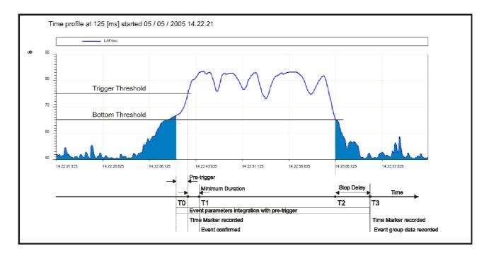
Fig. 8 - Description of the event trigger parameters
