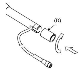
8. To secure the outdoor protection you can use the threaded end (D) or you can apply the fitting (E) on the tripod. The terminal (E) has two threads ,  $\frac{1}{2}$  " and  $\frac{1}{4}$ ".
