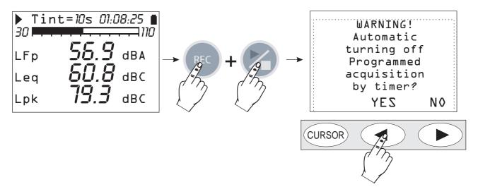
Fig. 12 - Delayed acquisition timer warning screen
