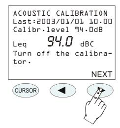
5. After the acoustic calibration, the **electric calibration** will be automatically started. This stage of the procedure generates the reference data for the following electrical calibrations.
