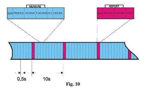
When the trigger function detects an event, identified by the overcoming of the trigger threshold, or when ENTER is pressed, a time marker is recorded.
