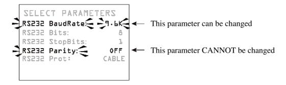
Press ENTER to access the selected submenu or to modify the selected parameter. Use the UP and DOWN arrows to edit the flashing selected parameter: press ENTER to confirm the new value, press MENU to cancel the input changes.
