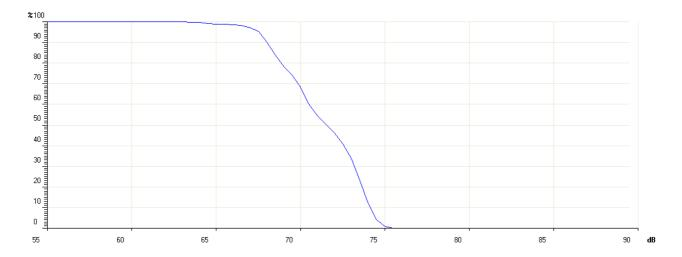
The cumulative probability will be null for levels higher than the maximum measured level. The percentile levels are calculated interpolating the cumulative distribution.
