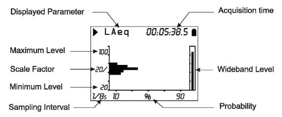
Fig. 6 - Description of the distribution of probabilities display
