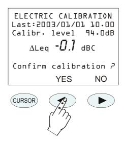
7. Press YES (keypad LEFT key) to confirm or NO (keypad RIGHT key) to refuse the calibration just finished. At the end, the instrument will switch to the SLM display, in STOP mode.
