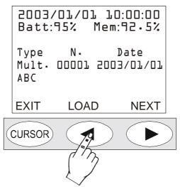
The following data are indicated for each file: the type (single, multiple or automatic), the progressive number given by the instrument upon logging and the date. Press NEXT to jump to the next file, press LOAD to download the current file.
