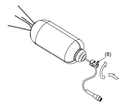
6. Insert the cable connected to the preamplifier through the system (C) and screw the stern to the support.
