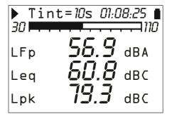
Before switching off the instrument, press STOP to end the ongoing measurement. If you do not do it, a message will request you to stop the measurement in progress: "WARNING! Stop the measurement to continue".
