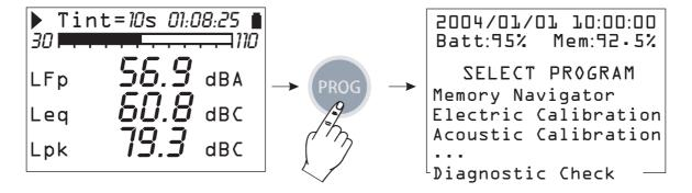
Use the UP and DOWN arrows to select the calibration to be carried out:
