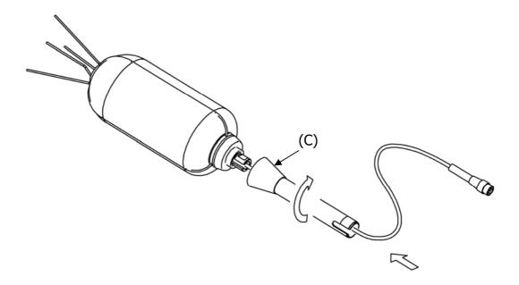
7. Screw the terminal placed at the lower end of the stern (D) releasing the cable laterally.
