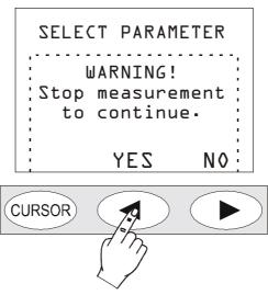
Press YES and then ON/OFF to switch off the instrument.
