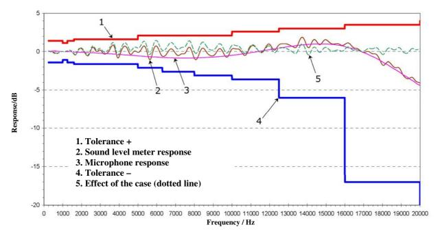
The selection of the UC52 microphones, on the basis of frequency response specifications, and the spectral corrections calculated by the sound level meter DSP allows obtaining a Class 1 response according to IEC 61672. The HD2010UC is also available in the Class 2 version.
