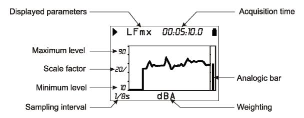
Fig. 5 - Description of the Profile mode display
