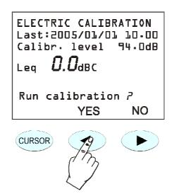
The screen shows date and time of the last calibration and the calibrator sound level according to the configuration of the respective parameter (MENU >> Calibration >> Calibr. Level). Answering positively to the request to continue, the selected calibration program will start.
