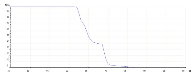
The *percentile levels* are calculated interpolating the cumulative distribution.
