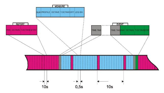
Fig. 11 - Recording flow for the Measurement, Report and Event groups
