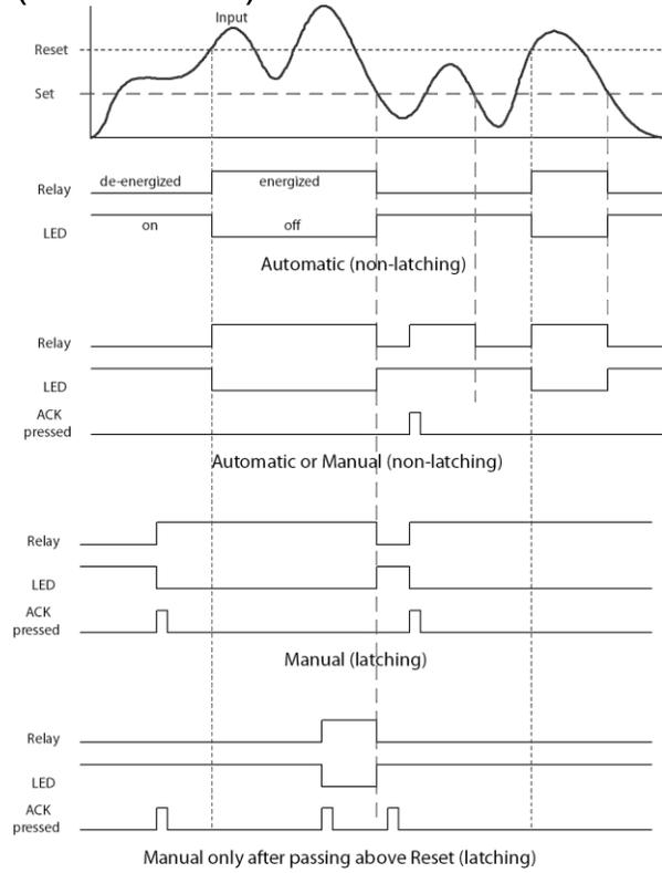
*Note: Relay coil is energized in non-alarm condition. In case of power failure, relay will go to alarm state.*
