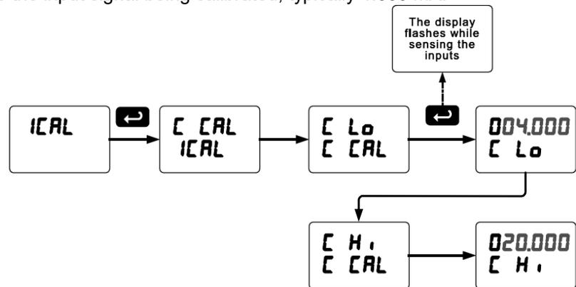
The graphic shows the calibration of the current input. The voltage input is calibrated in a similar way.
