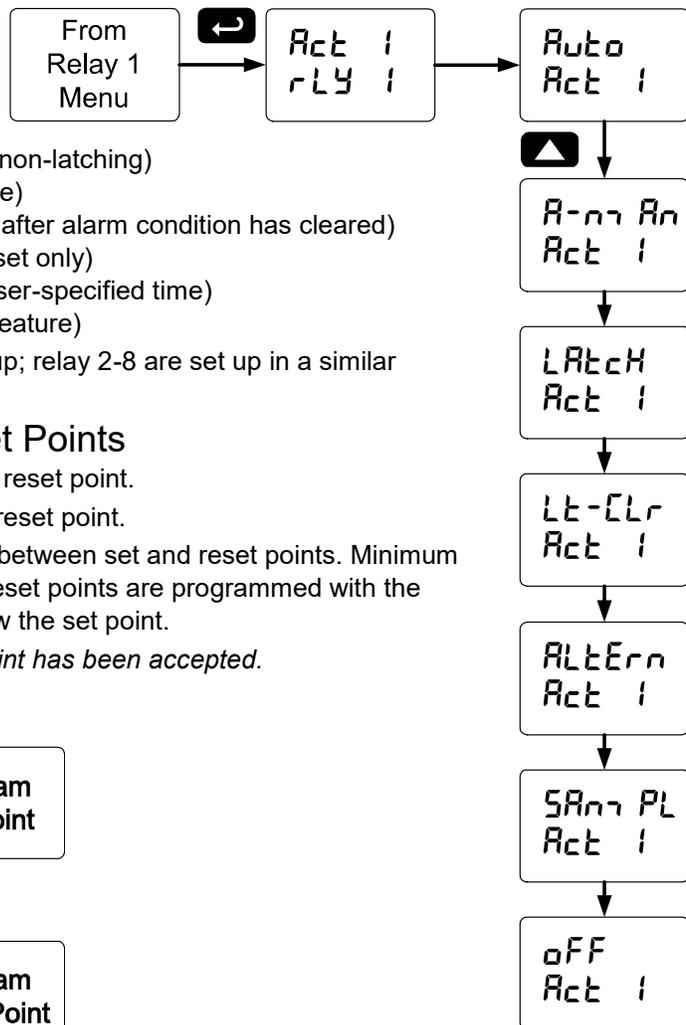
The following graphic shows relay 1 action setup; relay 2-8 are set up in a similar fashion.
