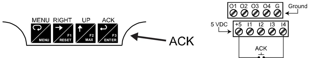
**Figure 23. Acknowledge Relays w/Function Key or Digital Input**
