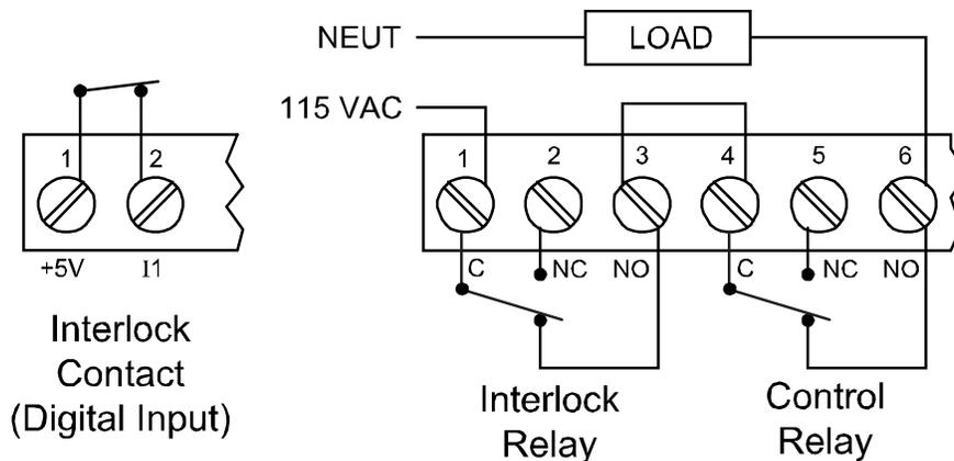
**Figure 22. Interlock Connections**
