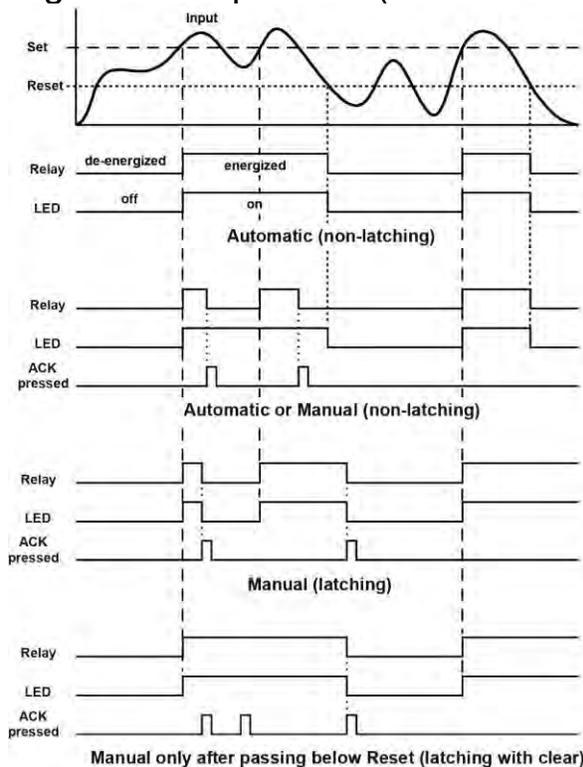
For Manual reset mode, ACK can be pressed anytime to turn "off" relay. To detect a new alarm condition, the signal must go below the set point, and then go above it.
