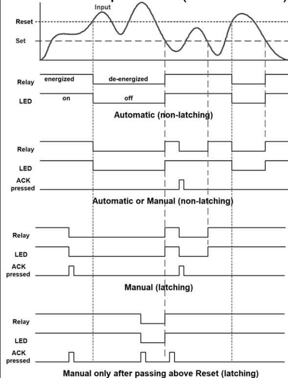
For Manual reset mode, ACK can be pressed anytime to turn "off" relay. For relay to turn back "on", signal must go above set point and then go below it.
