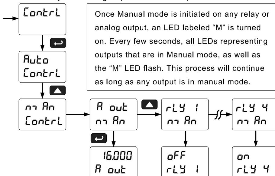
Once Manual mode is initiated on any relay or analog output, an LED labeled “M” is turned on. Every few seconds, all LEDs representing outputs that are in Manual mode, as well as the “M” LED flash. This process will continue as long as any output is in manual mode.
