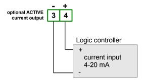
Figure 4.12. Example of current outputs connection (for device with current output only)
