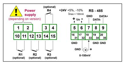
Figure 4.6. Terminals description (relay outputs, no current output version)
