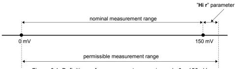
Figure 6.1. Definitions of measurement ranges in mode 0 ÷ 150mV
