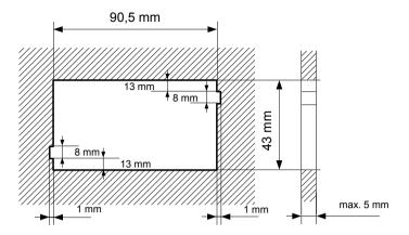
Figure 4.1. Recommended mounting hole dimensions
