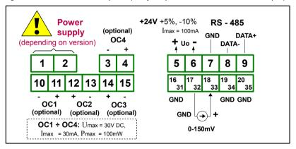
Figure 4.8. Terminals description (OC-type outputs)
