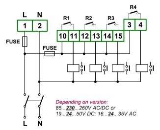
Figure 4.10. Connection of power supply and relays
