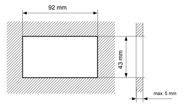
Figure 4.2. Allowable mounting hole dimensions
