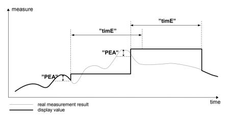
Figure 6.2. Process of peaks detection
