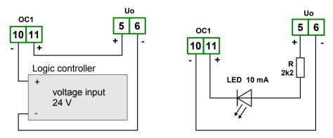
Figure 4.11. Example of OC-type outputs connection
