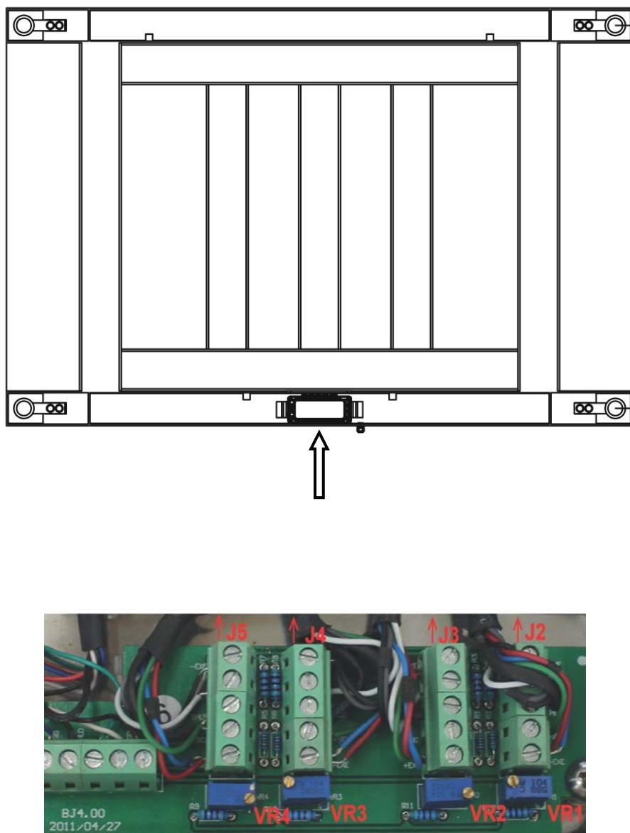
Adjustment of weighing cell J2 takes place at the potentiometer VR1.
